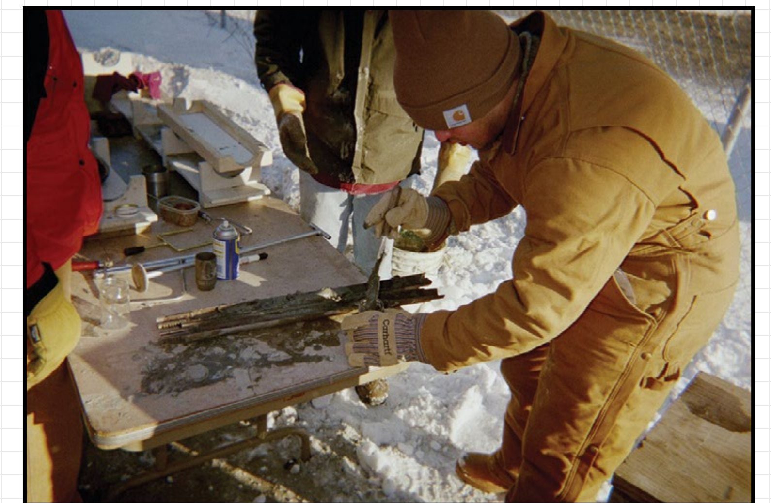
Typical collection of a soil sample from a split spoon sampling device
